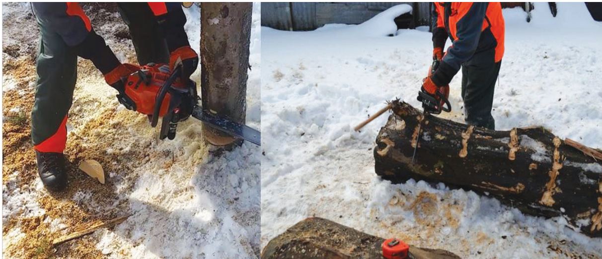
Fig. 1: Log positioning and simulations in the field. Legend: left - simulations on notch cutting on a vertically positioned log, right - simulations of bucking on a horizontally positioned log
