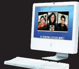
iMac Core Duo: 10 ianuarie 2006 Procesor: Core Duo 1,8/2 GHz, Video: ATI X1600, RAM: 512 MB, HDD: 160 GB, GigabitLan, Wifi 802.11g
