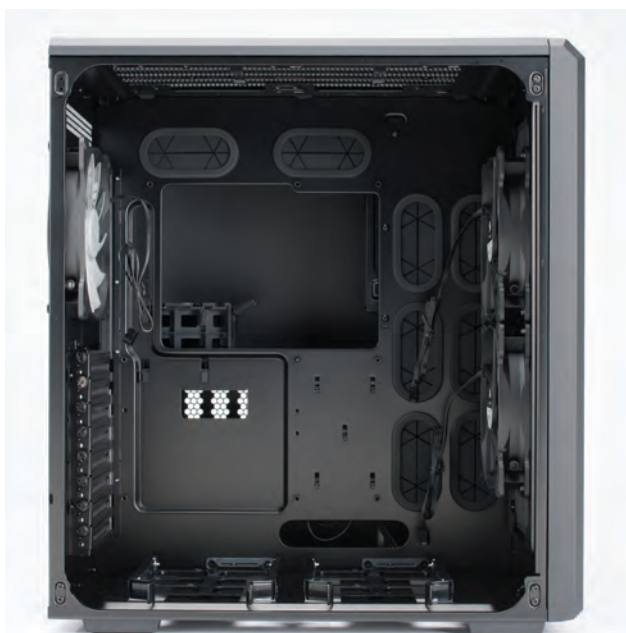
The left-hand “chamber” is eight inches wide, leaving five inches on the other side for the power supply and 5.25-inch drive bays.
