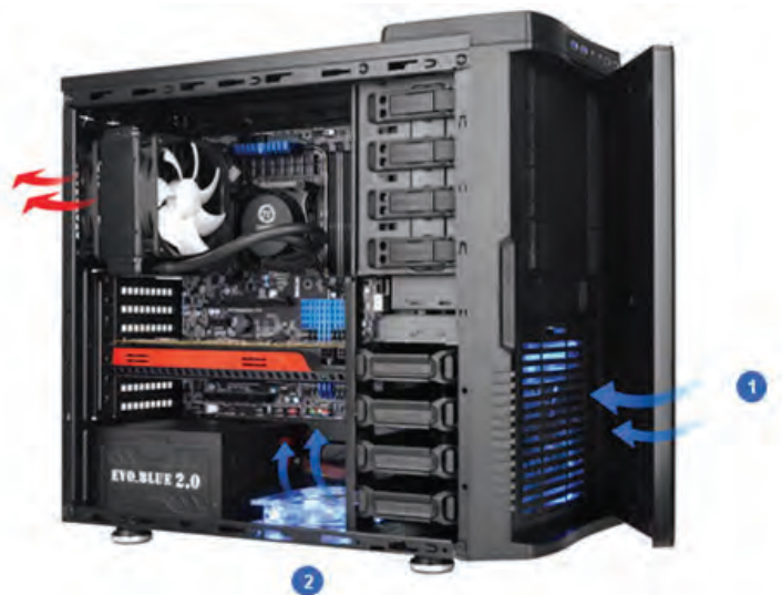
This photo from Thermaltake's website shows the standard placement for a closed-loop liquid-cooler's radiator.
