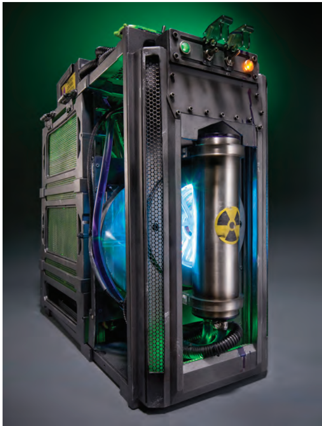
The Lanboy Apocalypse is a computer masquerading as a makeshift nuclear reactor. Lamborghini-style side panels open up to reveal a massive 250 millimeter fan that cools the Thermaltake radiator inside. Photo by Brian D. Garrity.
