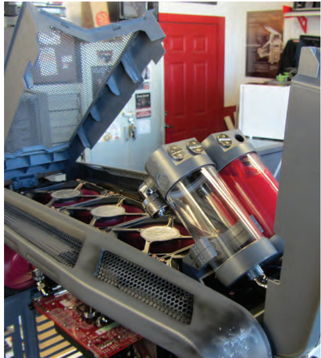
This Rebel Alliance-themed Cosmos II has two separate water-cooling loops for maximum performance. The distinctive red coolant is a custom mixture of Mayhems dyes cooled by two 480 millimeter radiators mounted on the top and front of the case. Photo by Bill Owen.
