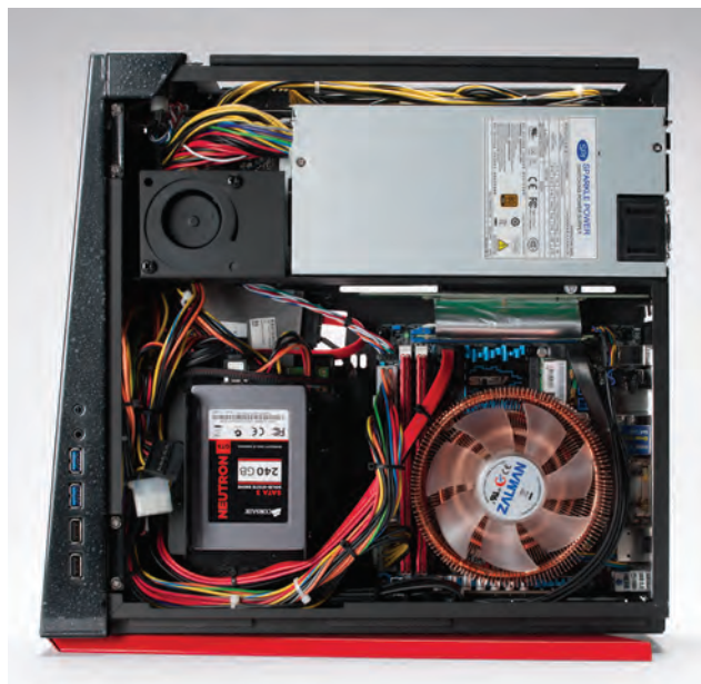
The Bolt's outer shell slides off to give you easy access to its guts, and there's even a cutout in back for the motherboard.
