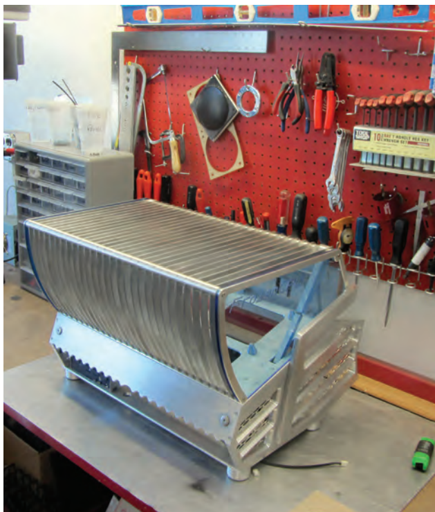
This scratch-built tech bench commissioned by FrozenCPU.com is made almost entirely of billet aluminum with a cover that opens automatically to reveal the components inside. Photo by Bill Owen.
