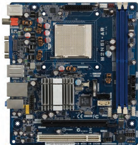
This Asus board, exclusive to some long-vanished HP mini-machine, has a proprietary power connector instead of the standard ATX 24-pin. Fortunately, adapters are available.
