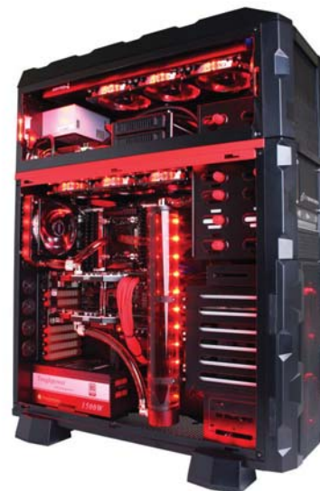
The Azza Fusion 4000 has room for an XL-ATX motherboard on the bottom and a Mini-ITX rig on top, perfect for your multiboxing needs.
