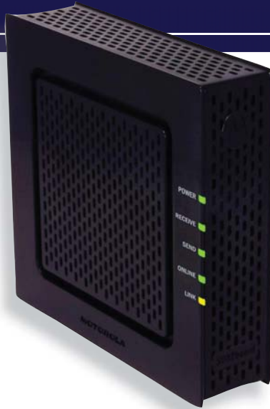
The Data Over Cable Service Interface Specification, or DOCSIS, is used by many cable television operators to provide broadband Internet access over their existing network using a cable modem, like the Motorola SB6120 pictured here.
