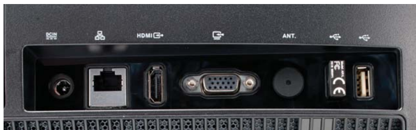
We were surprised to find a VGA input on the Asus ET2701's back panel.
