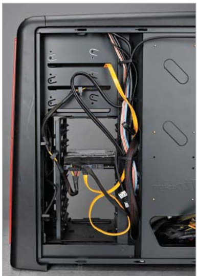
There's not much room behind the motherboard tray, but the Element S does provide for some cable-routing options between the mobo and drive trays
