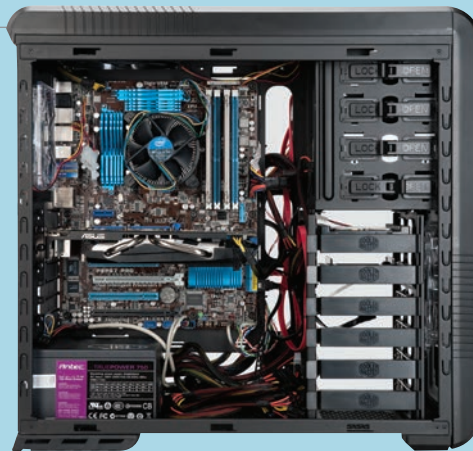
Sloppy wiring can create pockets of hot air and dust in your case.
