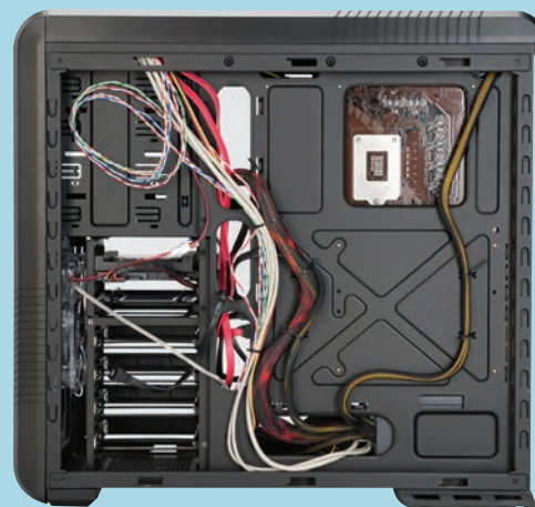
Sloppy wiring can create pockets of hot air and dust in your case.
