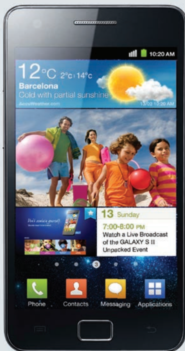
Samsung's own 1.2GHz Exynos 4210 dual-core processor makes an impressive debut in the Galaxy S II.
