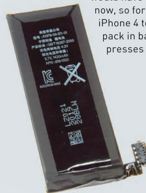
The iPhone 4's 1,420 mAh battery registers as relatively puny, meaning the phone runs quite efficiently.
