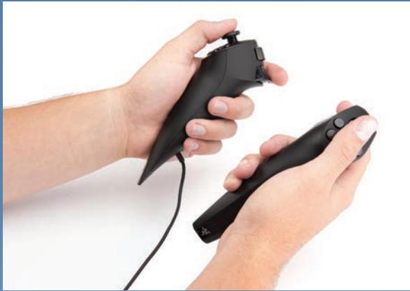
The Hydra's controllers are tethered to the sensor by hardwired cables.
