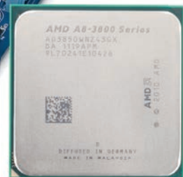
The A8 X4 3850 spends half of its transistors on graphics and it shows.
