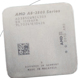
The A8-3850 combines a quad-core chip equivalent of an Athlon II X4 with the power of a discrete GPU.
