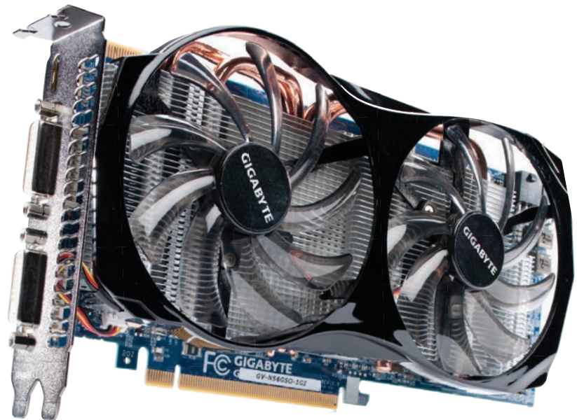
A second fan lets Gigabyte massively overclock the GeForce GTX 560.
