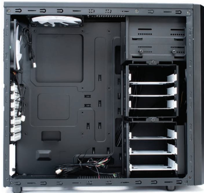
The Core 3000's top hard drive cage is easily removable to accommodate long videocards.
