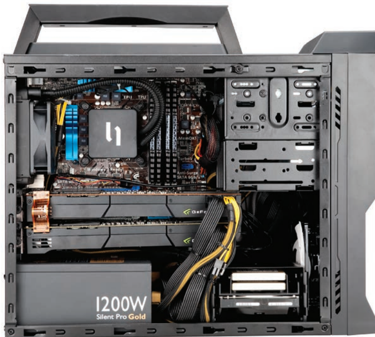
Air blown directly onto the GPUs seems to tame the noise of the GTX 590 cards.
