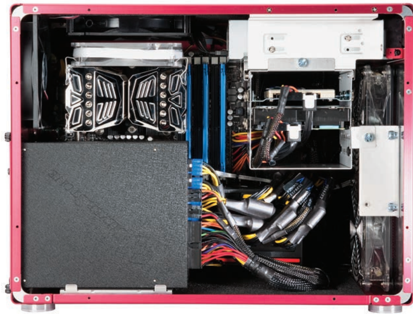
Tucked in behind the 1,200W PSU are two Radeon HD 6990 dual-GPU cards and a Prolimatech Megahalem.
