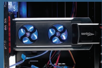
The two 8cm side intake fans cool the GPU area.
