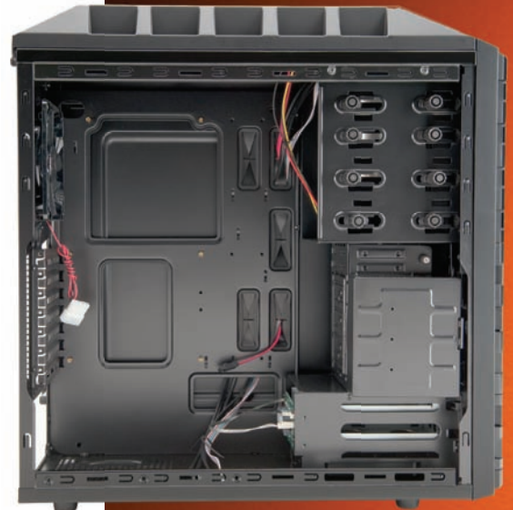
The five rubber-grommeted routing cutouts in the mobo tray make organization a snap.
