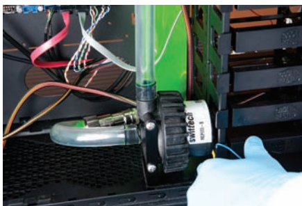
Fluid going... vertical? It has to happen at some point, because you always want your pump to be one of the lowest elements in the entire loop—good luck priming the darn thing otherwise.
