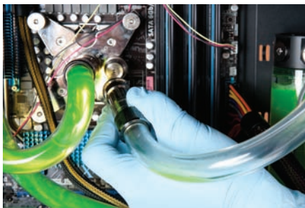
Koolance's Quick Disconnects meant we could literally remove and connect hoses at-will, fluid-filled or otherwise.
