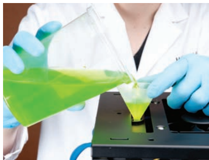
Now's a good time to remind you that the first real act of filling your fluid loop should happen outside of your case.
