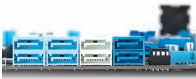
The SATA 3Gb/s ports on the Intel 6-series chipsets could fail over several years of use.
