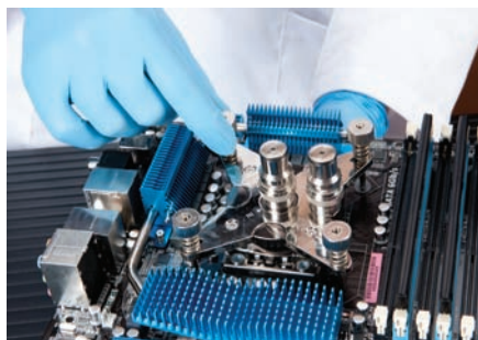
If you're going to use the same Koolance Quick Disconnects that we did, make sure the drilling of the water block's 1/4-inch holes are compatibly placed.
