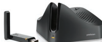
The Veebeam HD uses Wireless USB to stream HD video from your notebook PC to a television in the same room.
