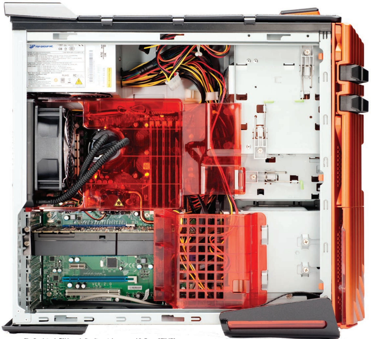
The Predator is "SLI-ready," so it can take a second GeForce GTX 470.
