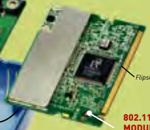
CPU The FV1000 controller chip is based on the ARM9 processor; it handles the bulk of the workload.
