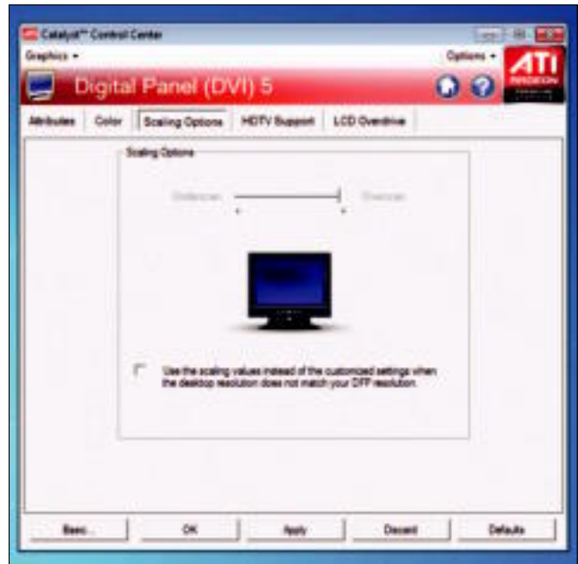
It's hard to find, but ATI's Catalyst Control Center does have an underscan/overscan slider.
