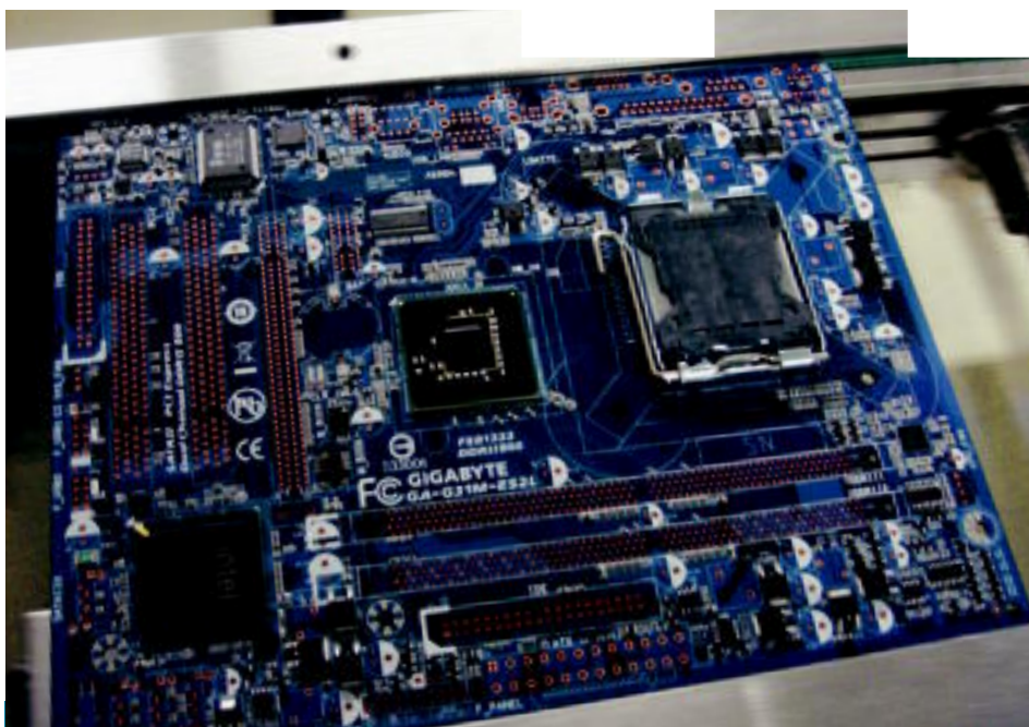
Here’s the result after the high-speed and multifunction placers have done their job.
