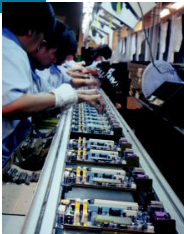
Every single PCI-E slot gets mounted by hand—remember that the next time you install a new GPU.
