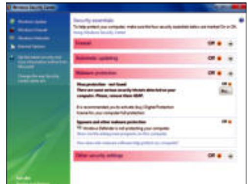
If you see this screen (as we did after CA ISS failed to protect our test bed), then something has gone terribly wrong. The real Windows Security Center will never direct you to a paid security suite.
