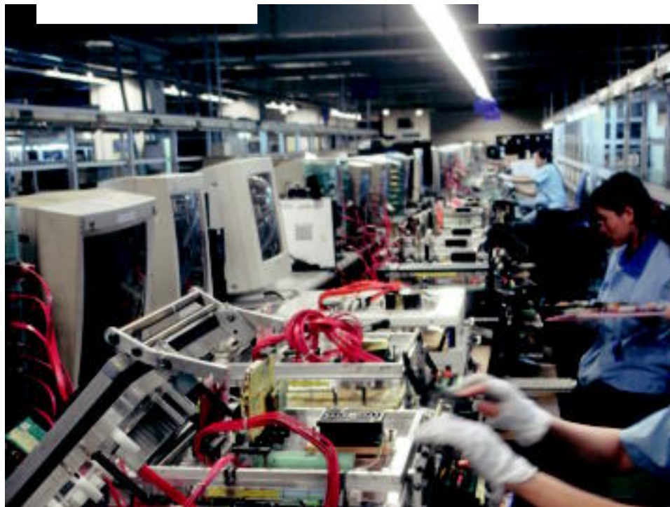
At a row of in-circuit testing benches, Gigabyte workers verify the electrical integrity of the newly placed components.
