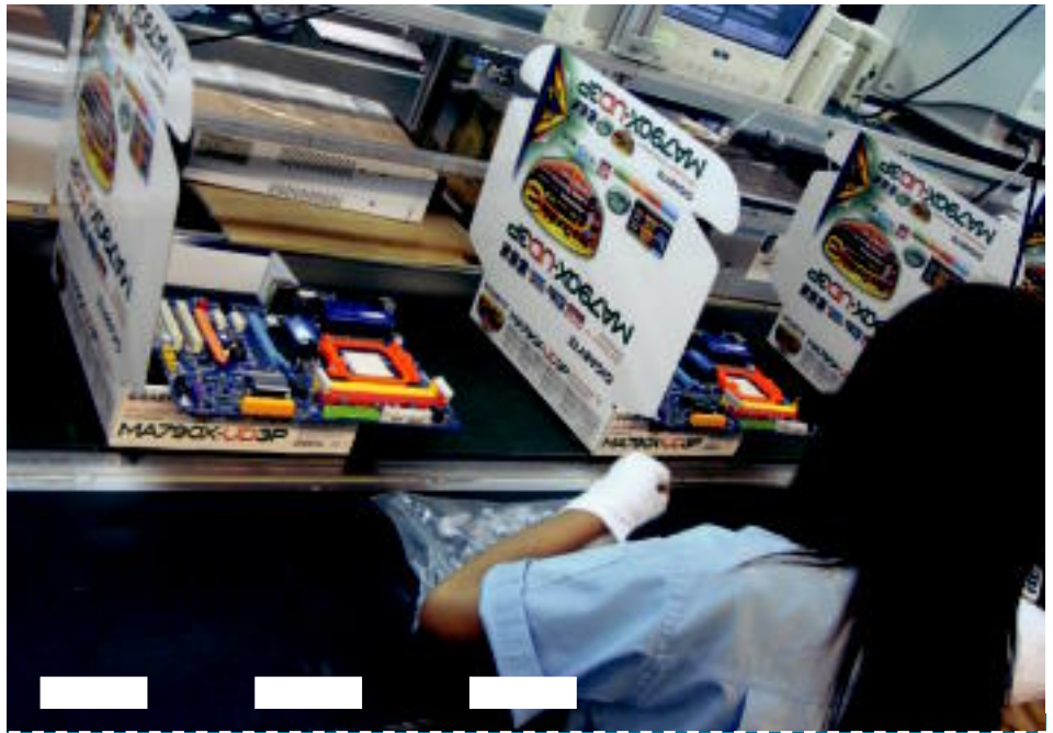
Within 15 minutes of first entering the assembly line, the once-bare printed circuit boards are now fully operational mobos, ready for retail.
