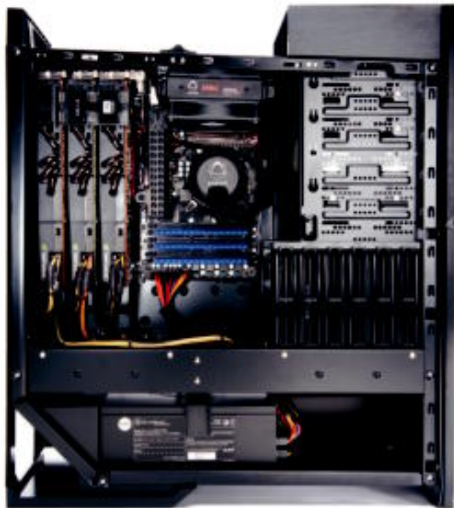
Maingear's slick new custom enclosure inverts the three GPUs to aid in cooling.
