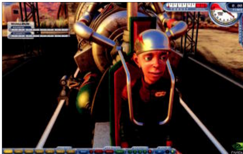
With hardware tessellation, character heads look properly curved, as do object like pipes.
