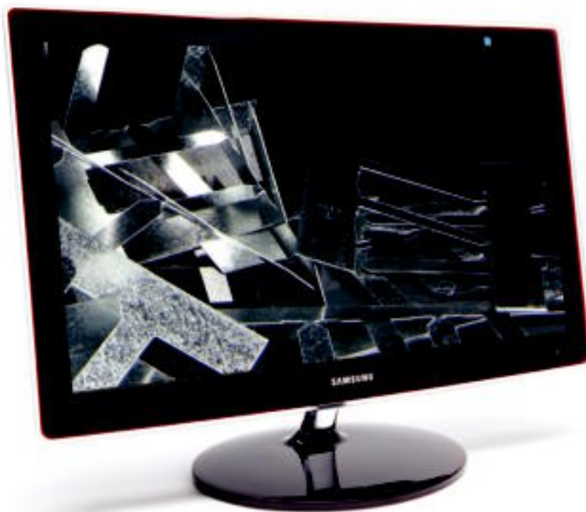
The Samsung P2770HD is a 6-bit TN panel, but Samsung maintains that its proprietary Hi-FRC frame-rate control enables it to display 16.7 million colors just like an 8-bit IPS model.
