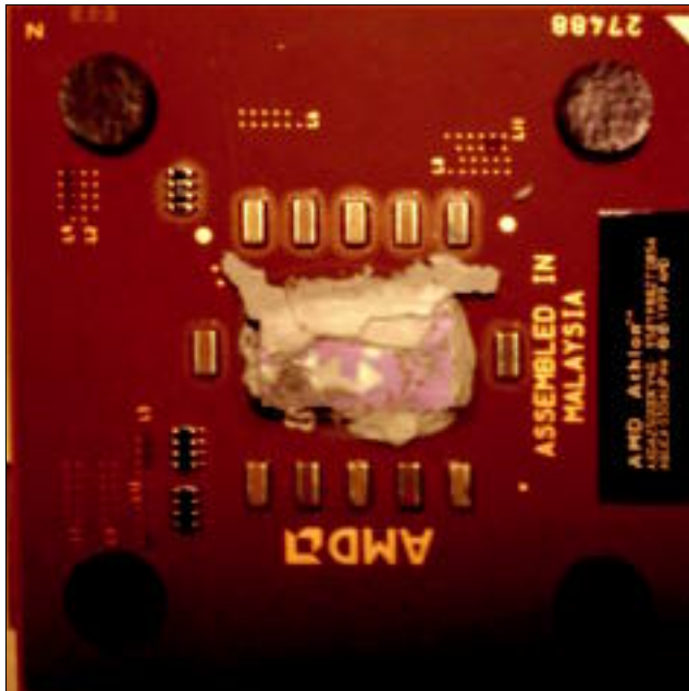
Be careful when cleaning CPUs that don't have heat spreaders—they're surprisingly easy to break.
