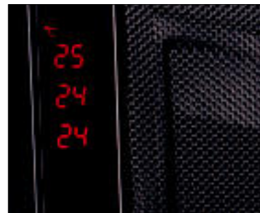
The three temperature displays on the front-panel LCD connect directly to three interior sensors.
