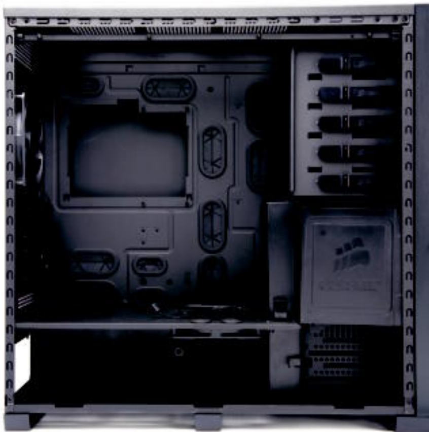
The case interior is roomy and packed with cable-routing cutouts. Wiring up a clean-looking case is almost too easy.
