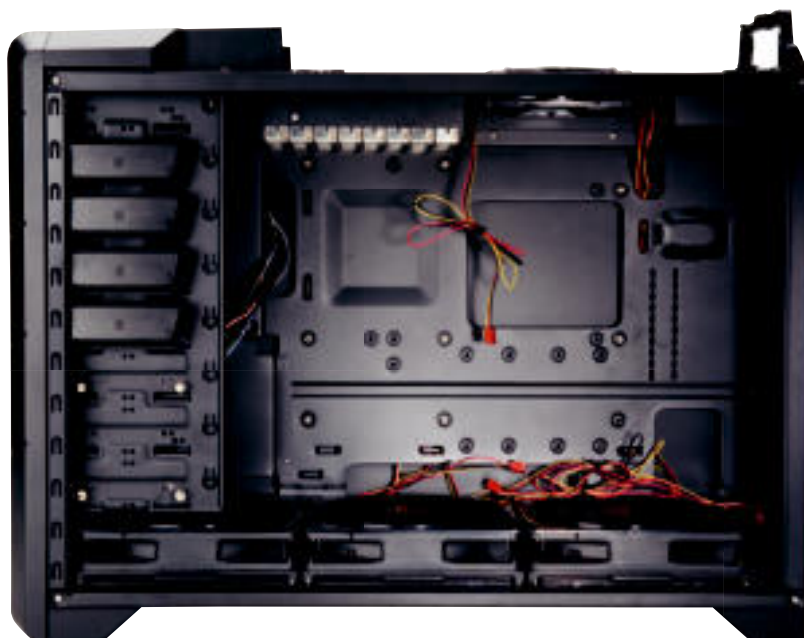
The Raven RV02's motherboard placement simplifies everything, from cable routing to airflow.
