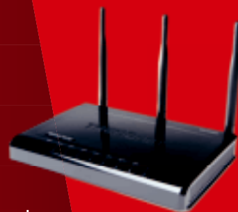
Trendnet's TEW-639GR single-band 802.11n router, reviewed in our Holiday 2009 issue, delivered the best throughput in four of our six test locations, so we used it as our basis for comparison.
