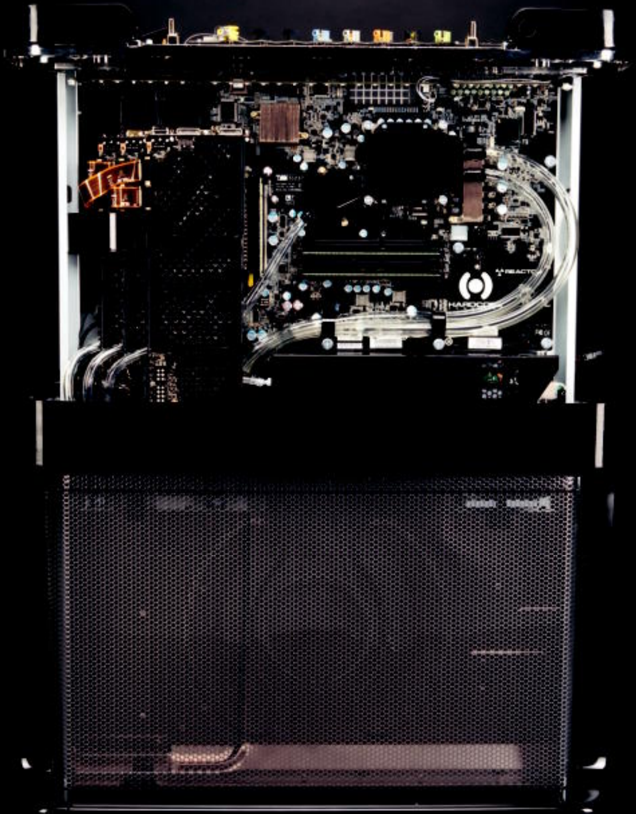
In operation, the Reactor PC's guts are submerged in a tank holding 4.5 gallons of dielectric mineral oil.
