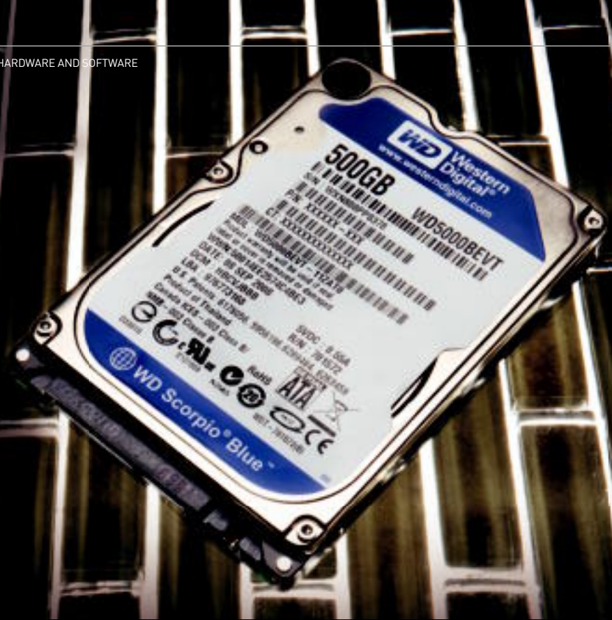
Western Digital's Scorpio Blue uses just two platters to reach 500GB.
