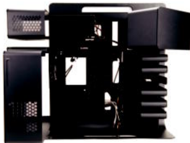
Clockwise from upper left: PSU compartment, optical drive compartment, hard drive bays, and motherboard compartment.
