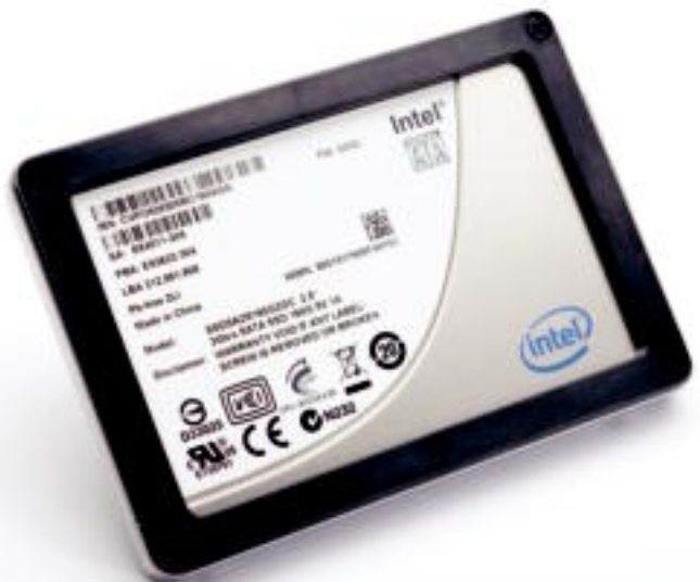
Many SSDs, like Intel's second-generation X-25M SSD, support the TRIM command, but the company's first-generation SSDs don't.
