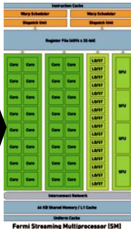
Fermi's streaming multiprocessors represent the most granular self-contained blocks, which will be used to engineer actual chip products.
