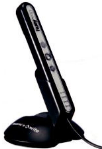
A color calibrator like the Pantone HueyPro will help match your monitors' color temperatures, even if they're from different manufacturers.
