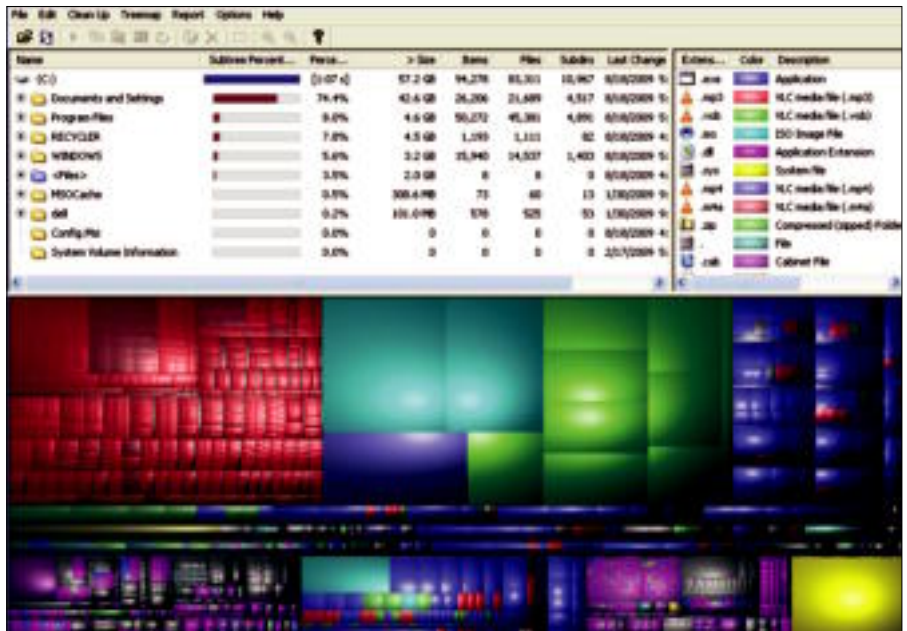
Graphical drive-space utilities like WinDirStat (shown) and SpaceSniffer let you see at a glance exactly which files are taking up precious hard disk space.
