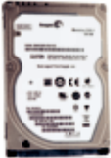
Seagate's Momentus 7200.4 is speedy, roomy, and only drains the battery a tad faster than a 5,400rpm drive.
