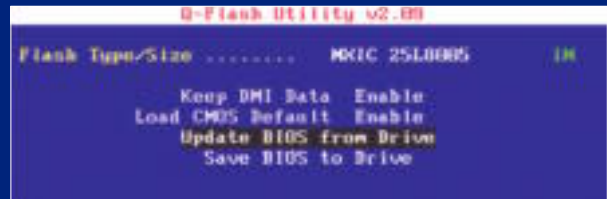
Gigabyte's Q-Flash utility walks you through the process of updating your BIOS.
