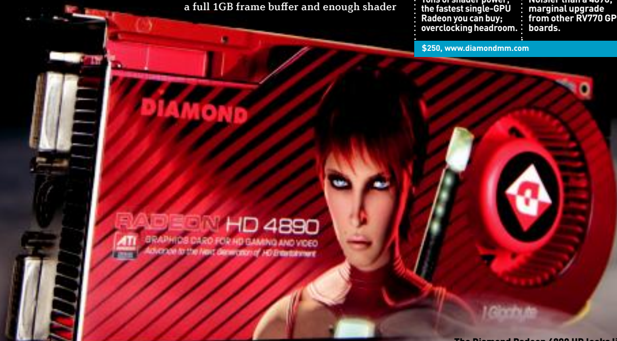
The Diamond Radeon 4890 HD looks like a stock card, but both its GPU core and GDDR5 memory are factory overclocked.
