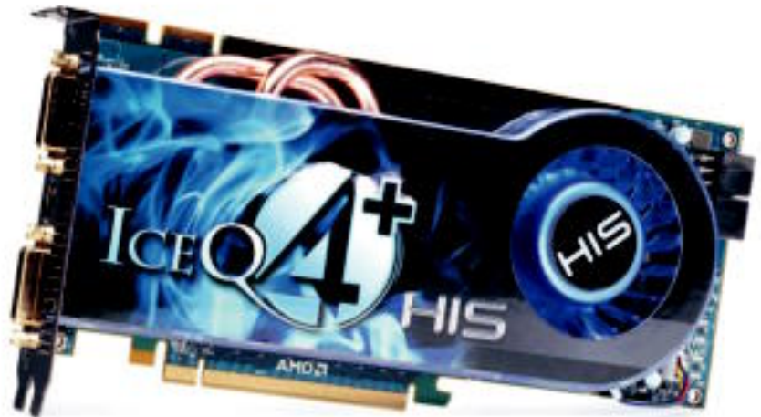
HIS put two dual-link DVI ports and an S-Video output on the mounting bracket; you’ll need a DVI-to-HDMI adapter to connect to a digital home-theater system.
