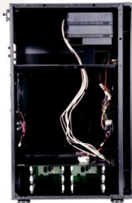
You gotta keep ‘em separated: This case keeps its hard drives far from the power supply.
