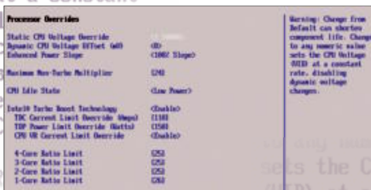
Extreme Edition CPUs feature unlocked QPI and memory override the individual Turbo Mode settings and change how the CPU throttles under power loads—to either run higher overclocks or
