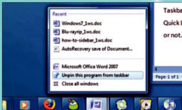
Jump lists give app developers a way to show context-sensitive information about their apps directly on the Taskbar. For example, Word displays a list of recently accessed files.
