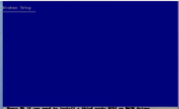
Blink and you may miss the F6 prompt during Windows XP's install for third-party drivers such as RAID, AHCI, or SCSI.
