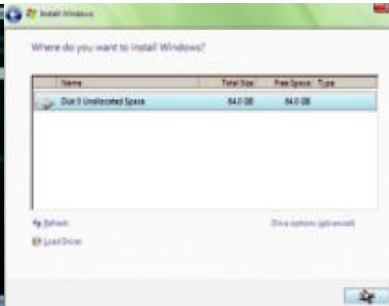
Most people will be suited by using one single contiguous partition for the OS, so just click next and Vista will format the drive that way.
