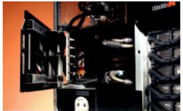
Close this swing-out panel and its spring-steel strips will push installed PCI Express cards firmly into their slots.
