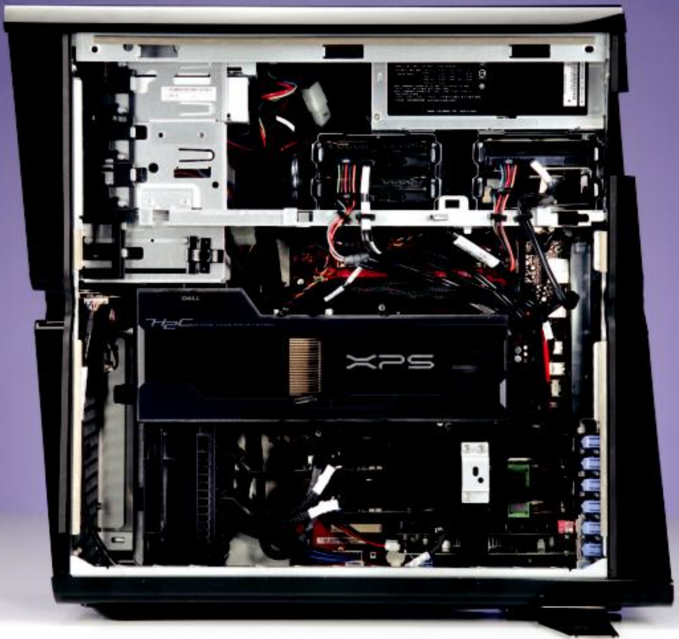
The H2C cooler dominates the 720's case, but there's still room for two 8800 Ultras, an X-Fi soundcard, and a PhysX card.
