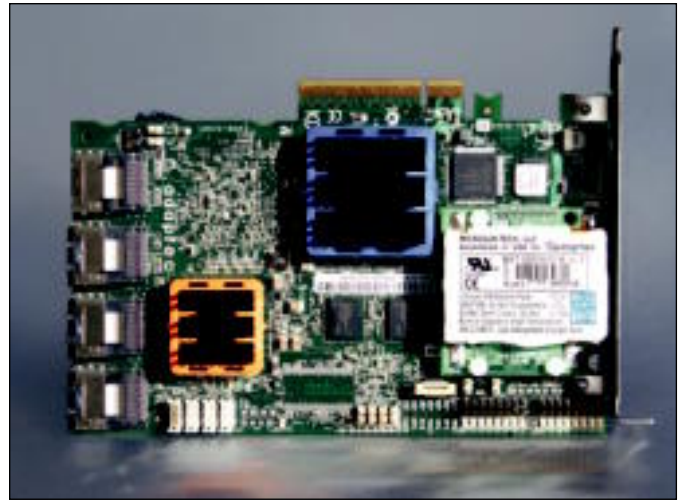
Adaptec's 31605 RAID controller costs a cool thousand bucks. But even it supports very few of the lesser RAIDs—only RAID 6, in fact.
