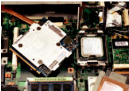
Don't rub your eyes, you're seeing an LGA775 desktop socket in a notebook and a user-changeable graphics card.
