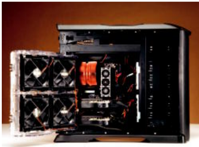
The heatsinks on the EVGA Ultra cards forced Project War Machine to 86 the soundcard.
