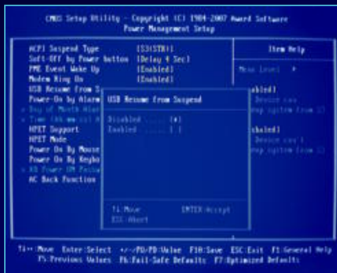
If a connected USB device sends signals to your PC nonstop, you will need to disable the USB Resume from Suspend option in your BIOS.
