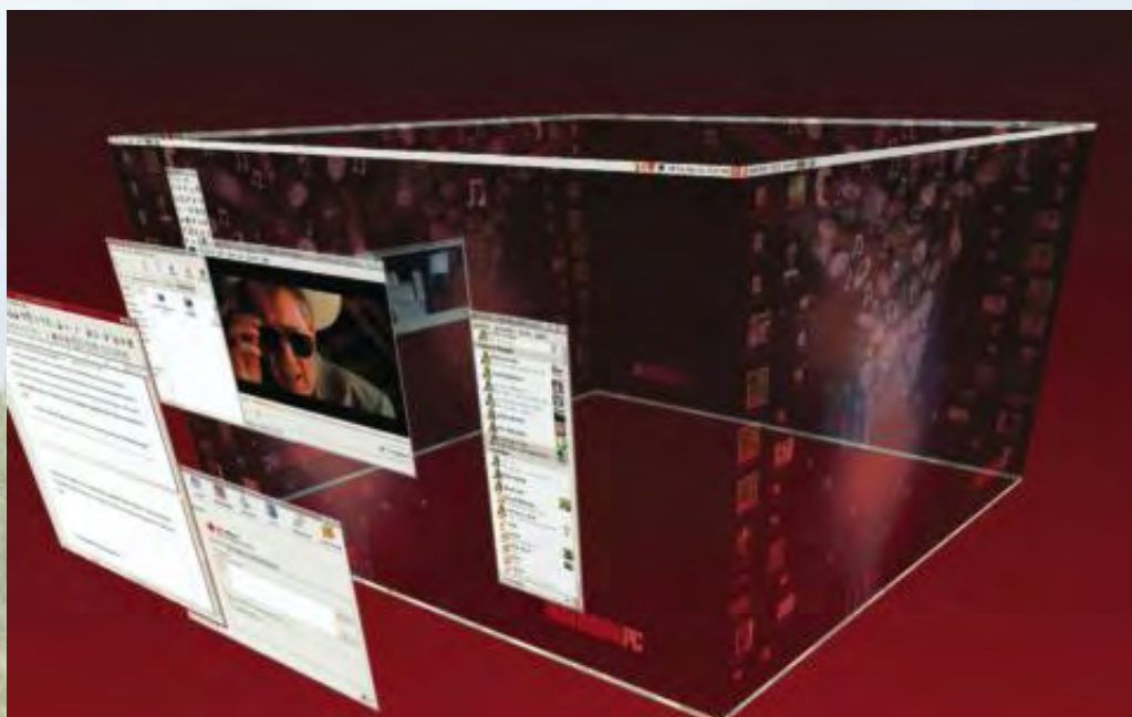
Beryl lets you map your virtual desktops to the outside of a cube, it's the next best thing to multiple monitors. (P.S. You can download the kick-ass wallpaper at www.maximumpc.com .)
