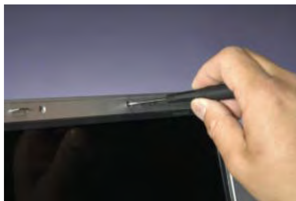
Step 1: Unscrew the bezel.
