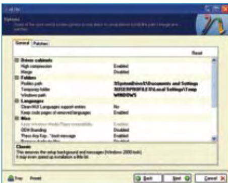
The Options and Patches window lets you alter the Windows install directory and USB mouse timing.
