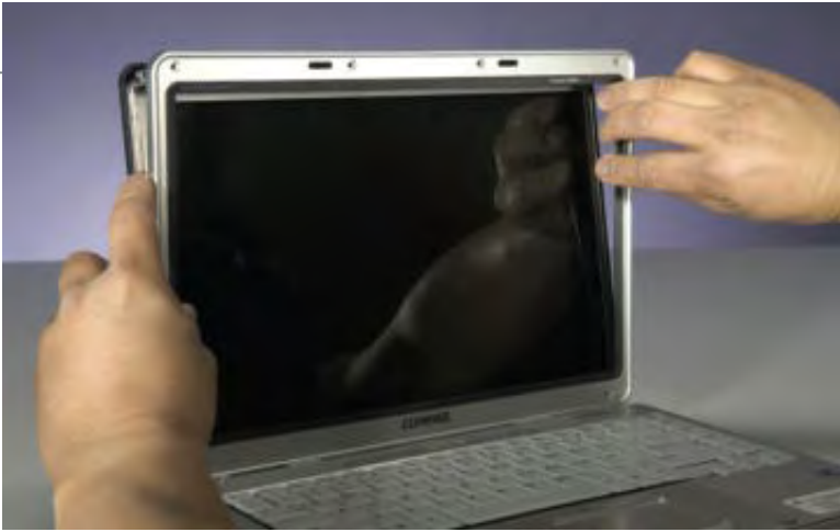
Step 2: Pry off the bezel.
