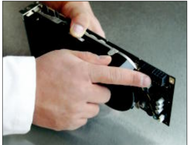
An early engineering-sample GeForce 8800 GTX sports a six-pin connector as well as a new eight-pin connector.
