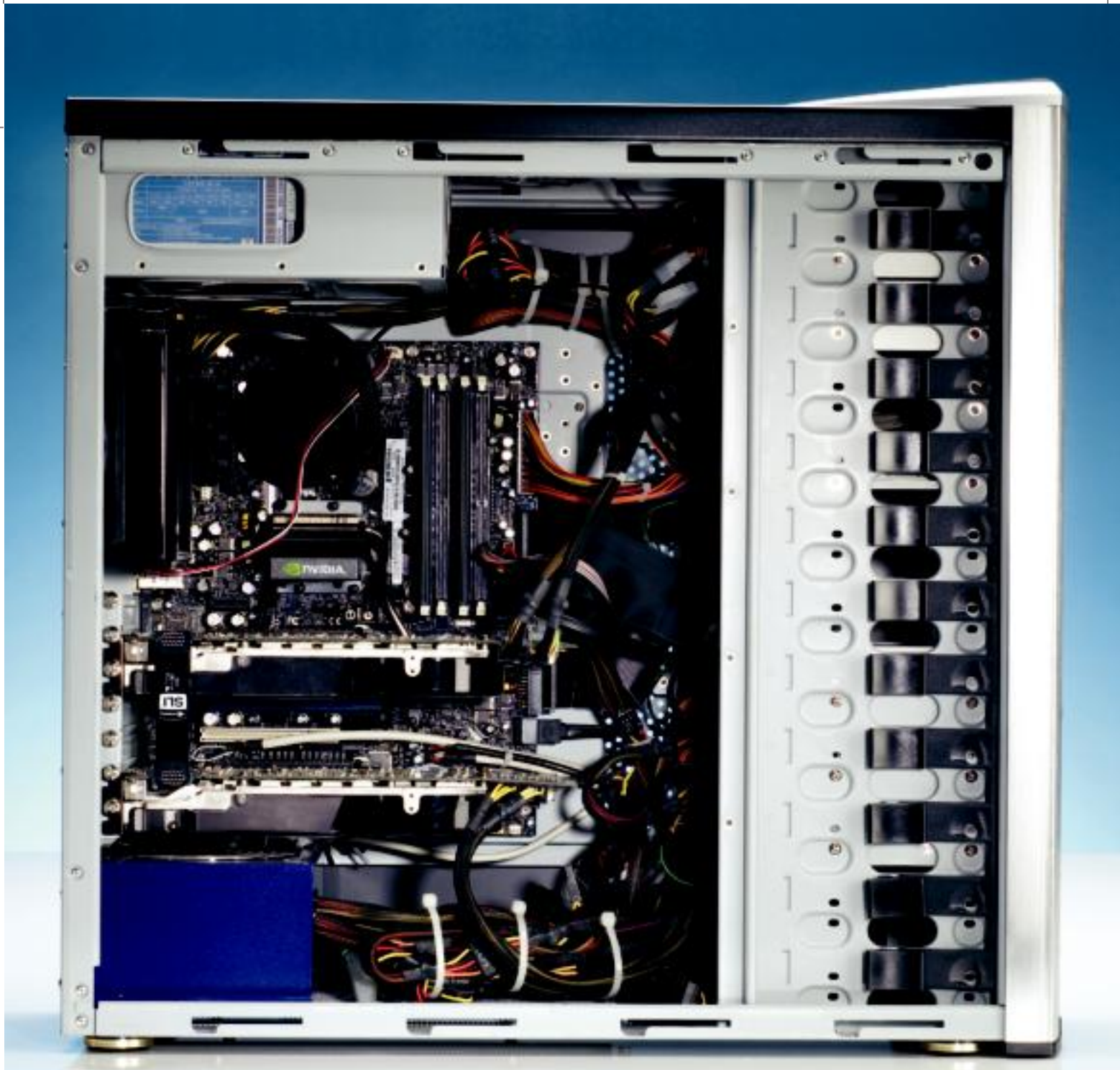
No need for a 1,000-watt power supply here; Polywell gives you two 700-watt power supplies.
