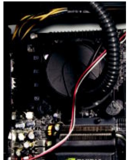
A new self-contained waterblock and cooler from Asetek doesn't require you to yank your mobo to remove the cooling.
