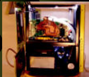
Khowdee used rivets to connect the two frames, then he fabricated a unified front panel out of aluminum and affixed it to the case with epoxy. After everything else was said and done, he applied multiple coats of sparkly Lemon Yellow Candy automotive paint.
