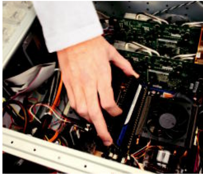
The four DIMM slots in the Quad FX platform feed two independent memory controllers in the CPU cores.
