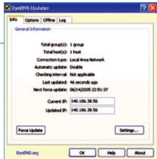
The free DynDNS service allows you to maintain the same URL for your website even if your ISP keeps giving your server different IP addresses.
