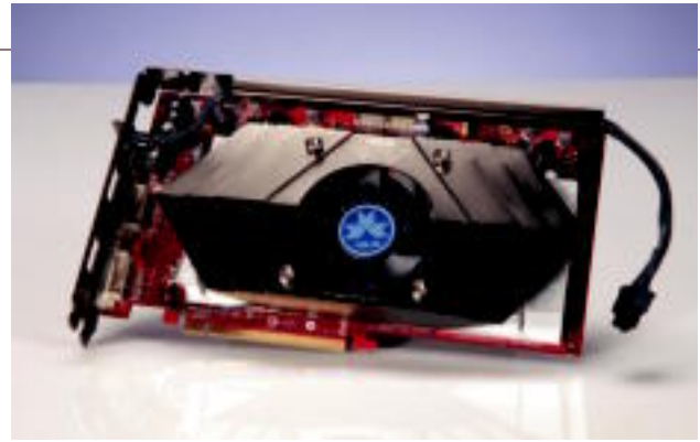
Asus' N7800GT Dual cleverly manages to squeeze two GeForce 7800 GT GPUs onto one circuit board. It delivers a sweet performance, but with a few strings attached.
