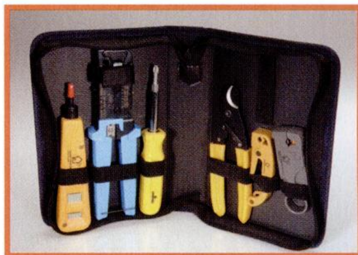
This network tool kit comes with cable stripper, crimper, and punch-down tool.
