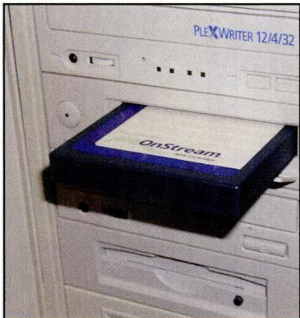
Slow SCSI tape drives on a faster SCSI chain won't slow the entire chain down at all times.
