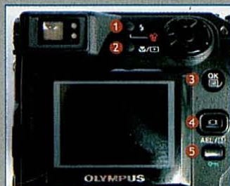
Butoane: 1 blitz 2 macro 3 meniu 4 monitor 5 protect
